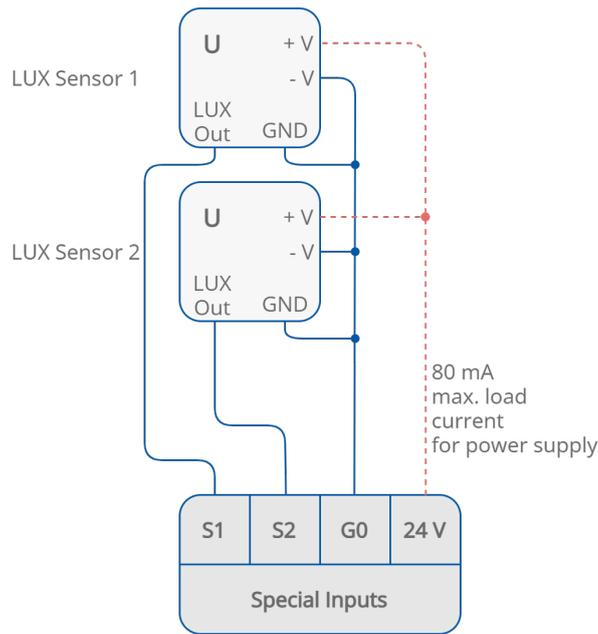
Figure 5. 24 V DC power supply connection
