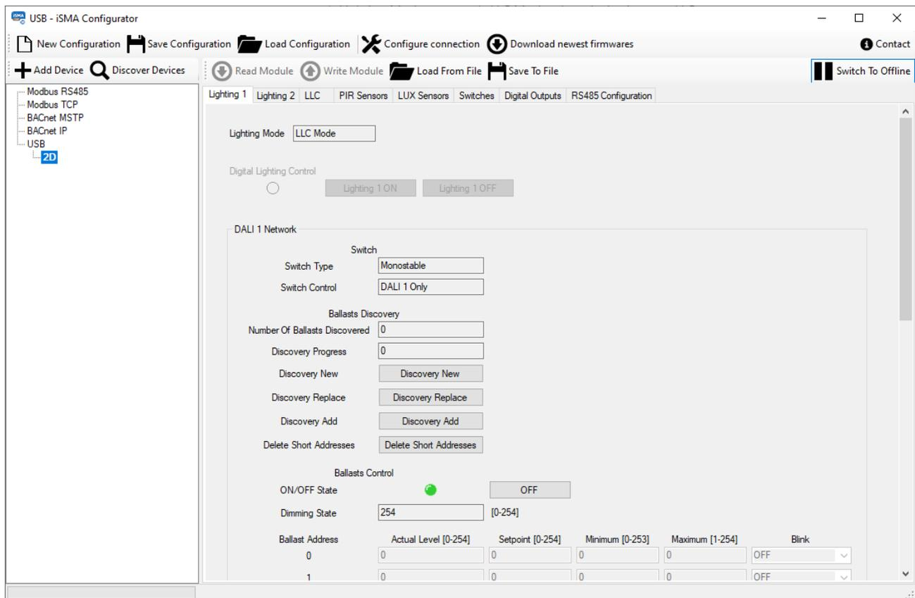
Figure 34. Lighting tabs 1 and 2 for devices working in the LLC mode
