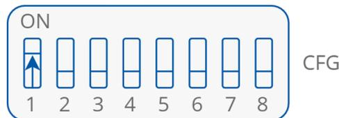
Figure 25. Bistable switch control configuration
