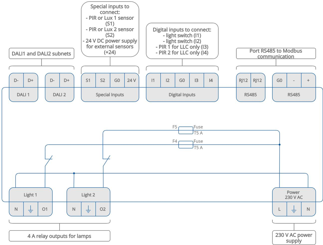
Figure 6. iSMA-B-2D-WD terminals and internal connections
