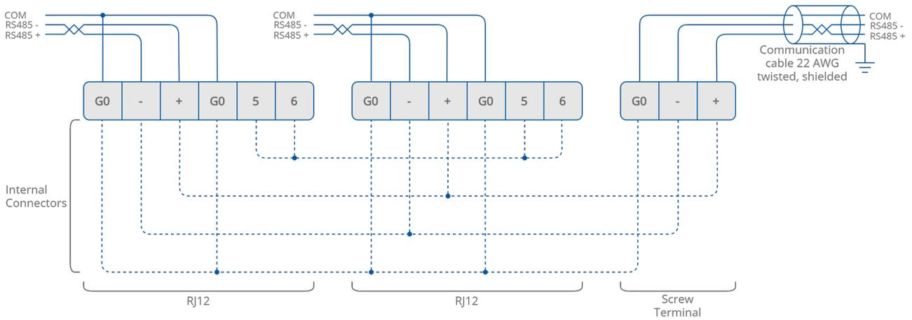
Figure 9. Internal connections between RJ12 sockets and a main RS485 socket
