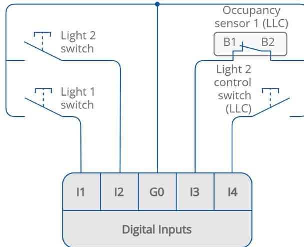
Figure 33. The light 2 control switch connected to I4
