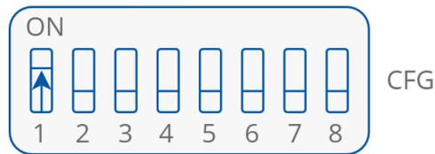
Figure 29. Bistable switch control configuration
