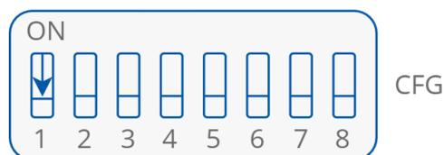
Figure 24. Monostable switch control configuration
