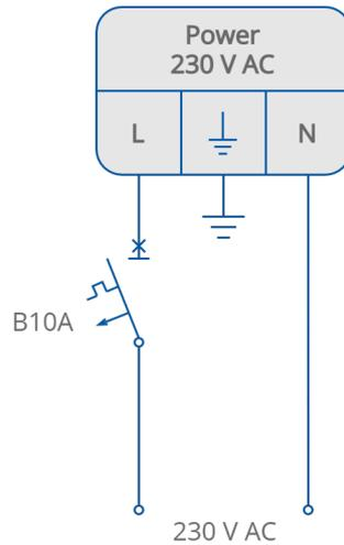
Figure 3. 230 V AC power supply connection
