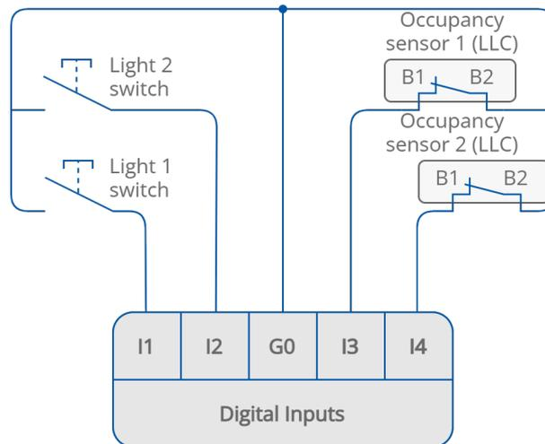
Figure 19. Connection of digital inputs dry contact
