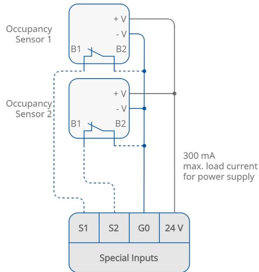
Figure 23. Example of connecting sensors to 24 V DC power supply outputs
