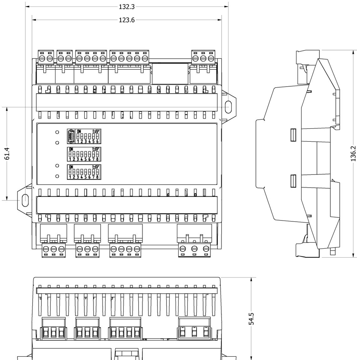
Figure 1. Dimensions of iSMA-B-2D
