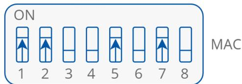
Figure 14. Setting an 83 address on the MAC DIP switch
