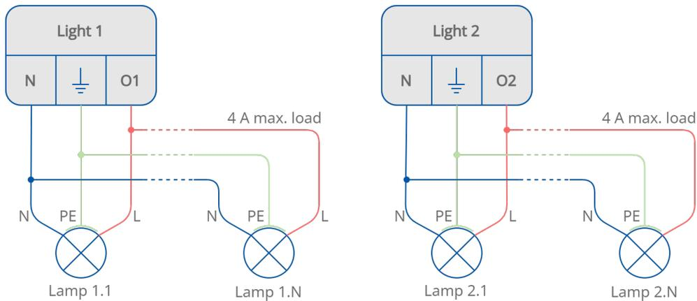
Figure 22. Connecting lamps to light outputs in the On/Off control mode
