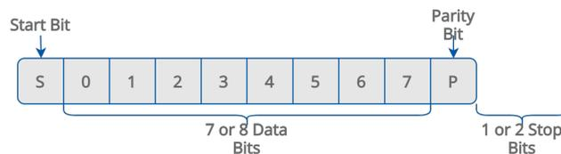
Figure 38. Modbus frame
