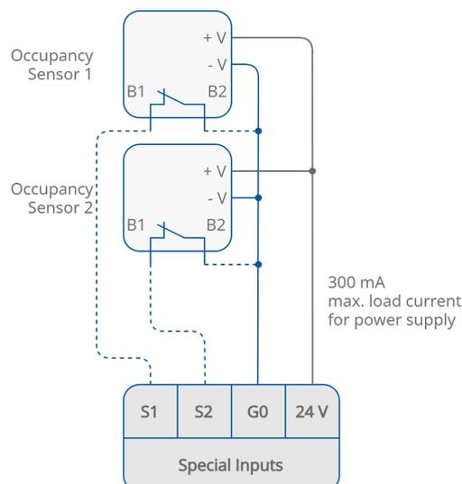
Figure 18. Special inputs connection
