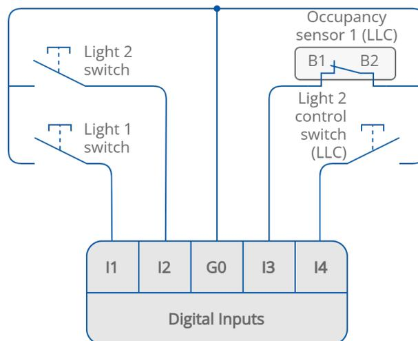
Figure 20. Connection of digital inputs with the light 2 control switch in the LLC mode
