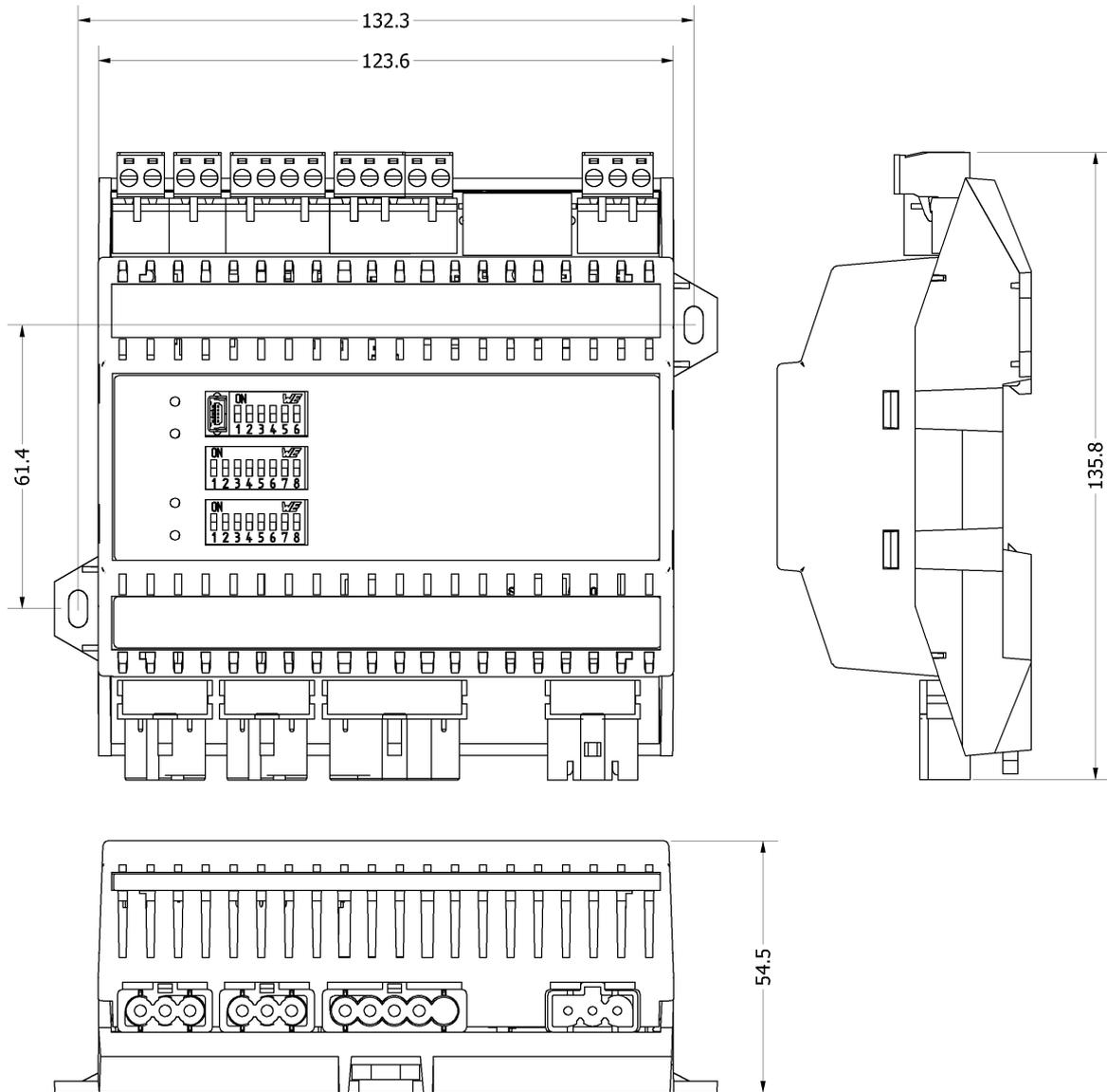
Figure 2. Dimensions of iSMA-B-2D-WD
