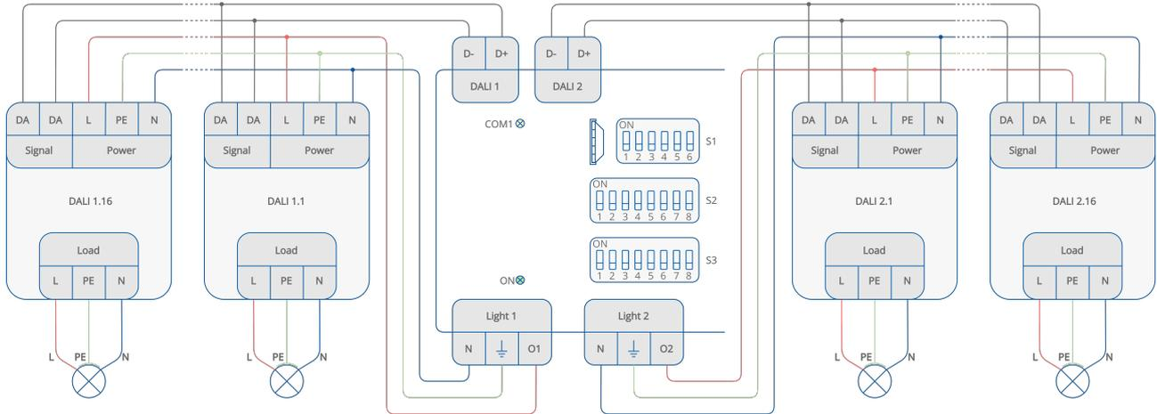
Figure 21. Connecting ballasts to light outputs in the DALI control mode
