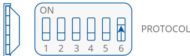
Figure 16. DIP switch for restoring default settings
