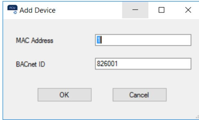
Figure 28. Adding a BACnet device manually
