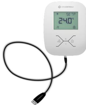
Figure 49. iSMA-B-LP panel USB connection
