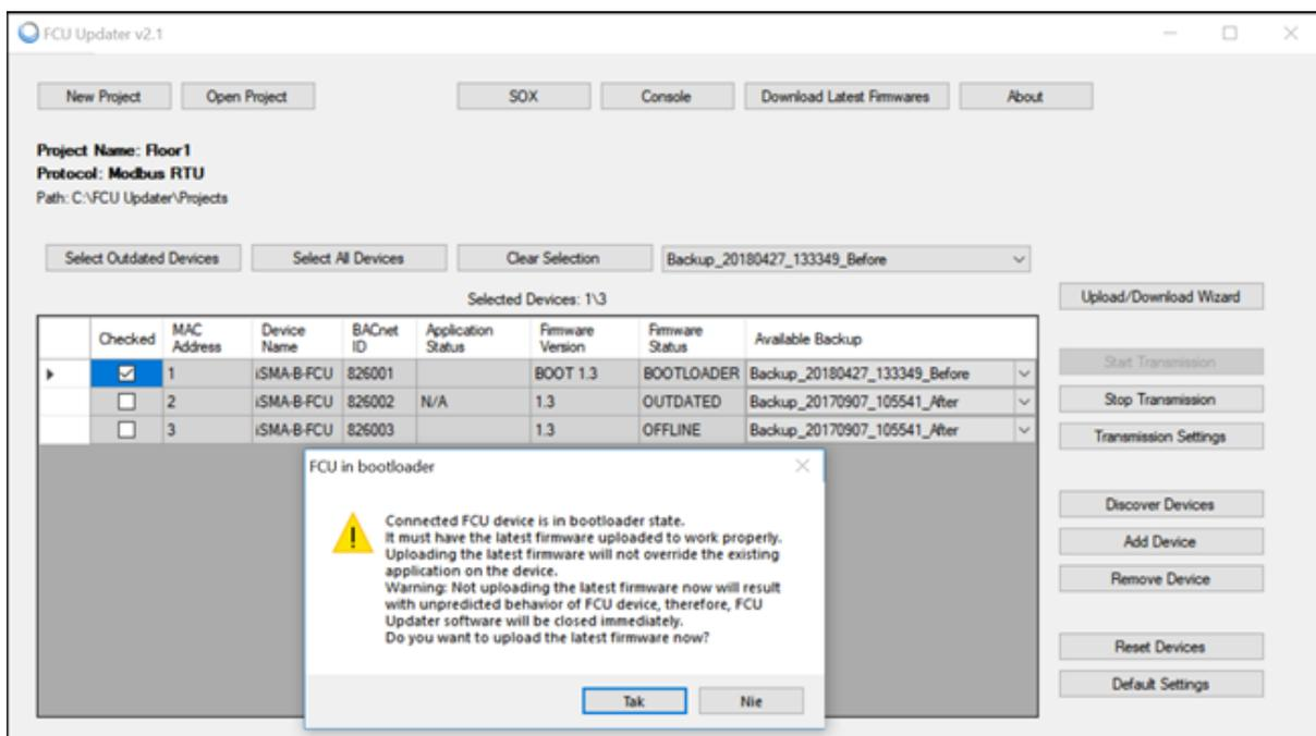
Figure 54. The FCU Updater recognizes a bootloader state in one controller
