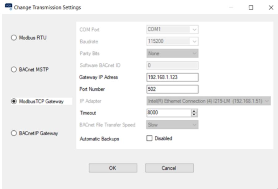
Figure 35. The Transmission Setting dialog window
