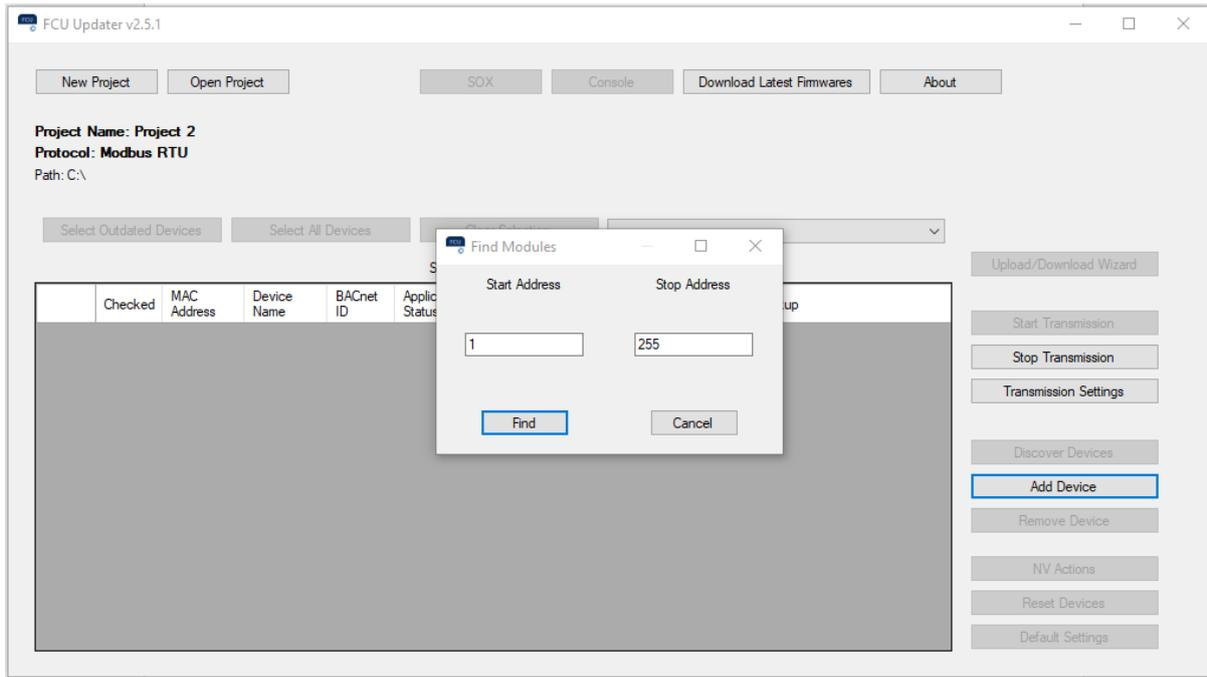
Figure 21. Discovering devices in the Modbus protocol
