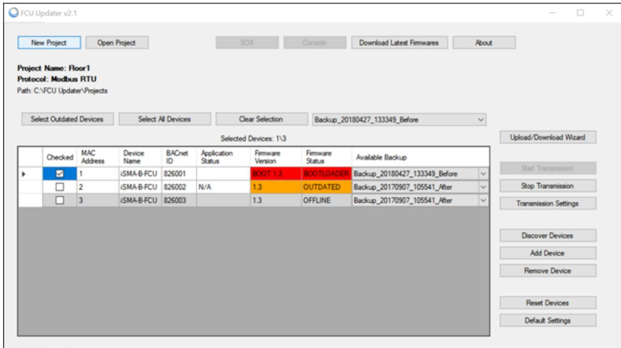
Figure 53. One of controllers in a bootloader state
