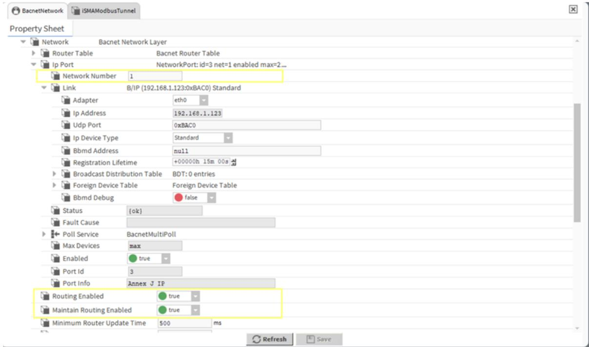
Figure 14. BACnet network settings required for the BACnet IP gateway to operate properly
