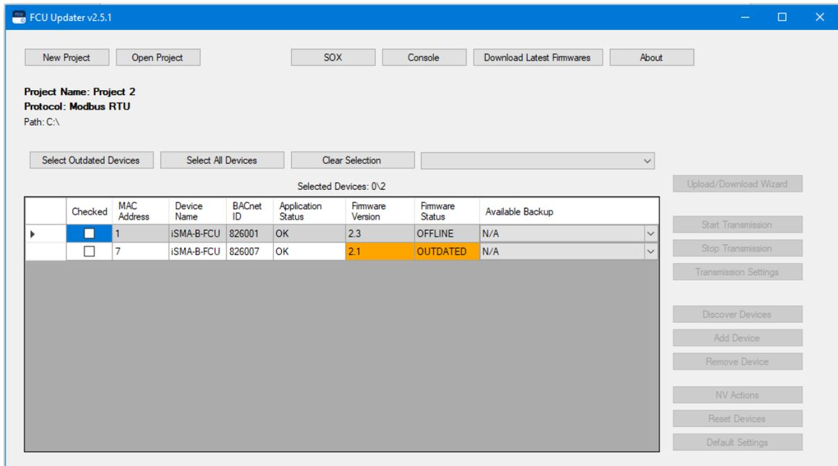
Figure 23. Discovered devices in the Modbus protocol
