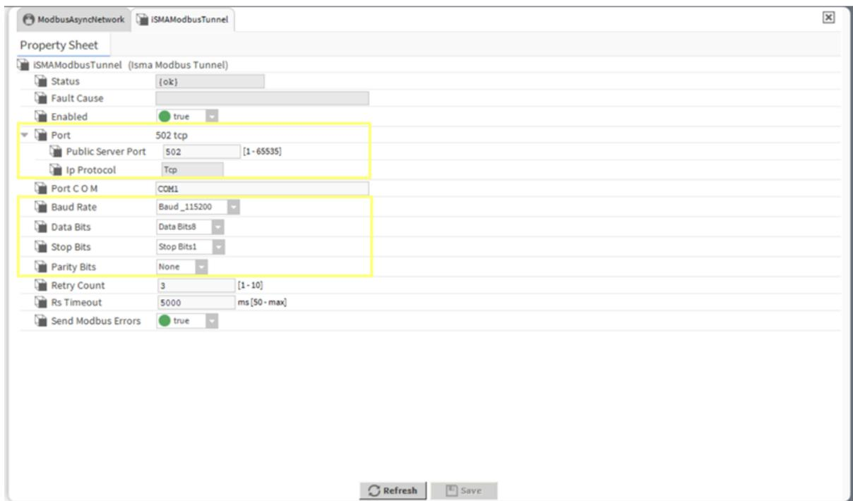
Figure 33. Communication parameters for the iSMA Modbus Tunnel
