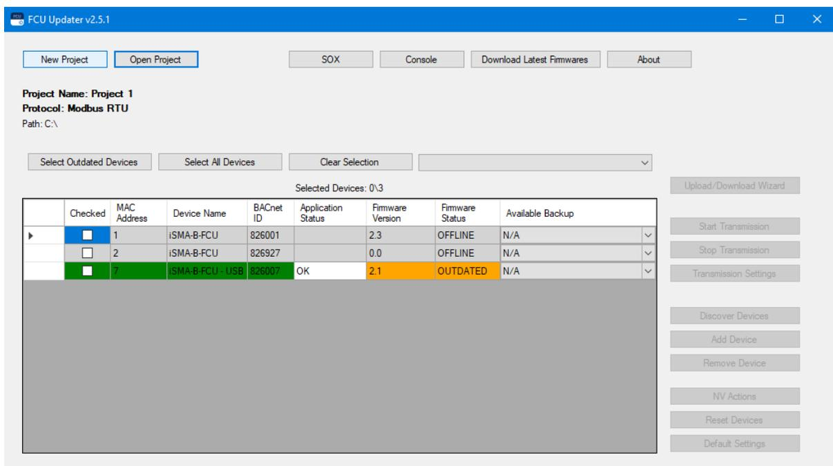
Figure 39. List with direct connections to devices with a USB cable
