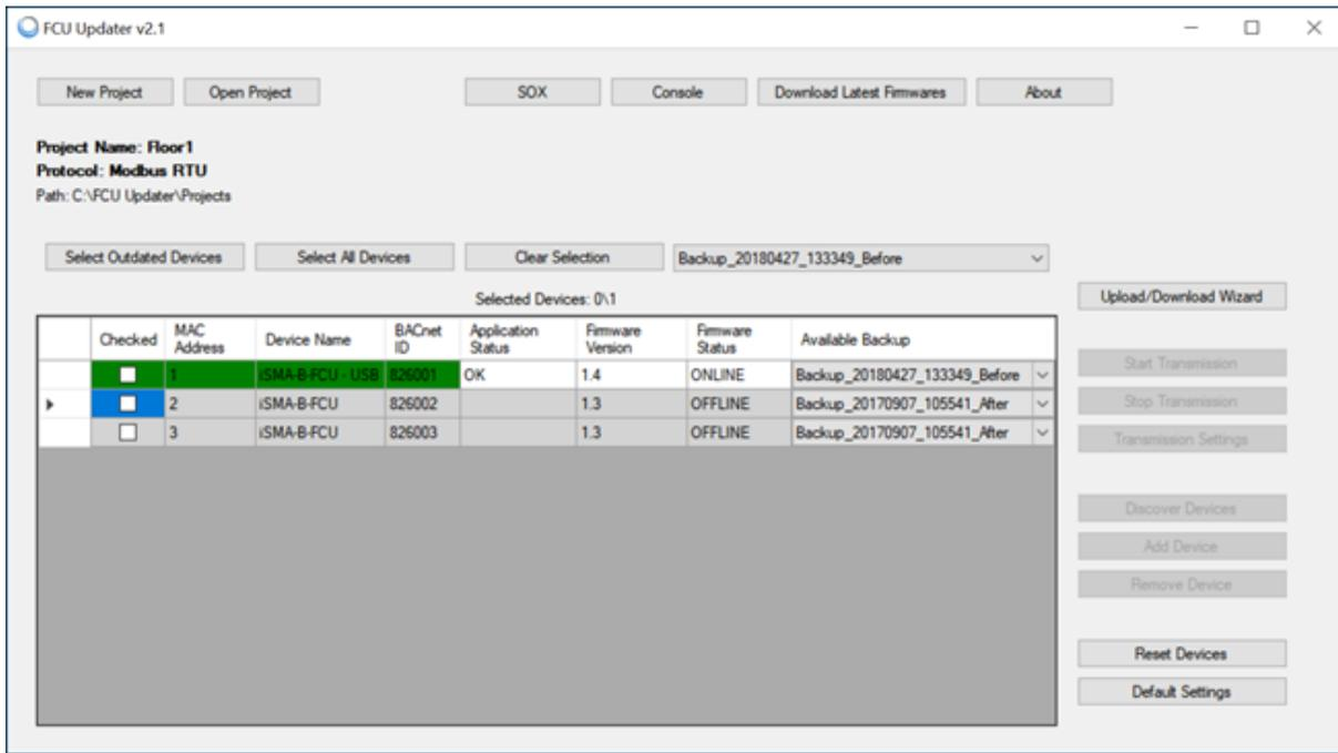
Figure 51. Directly USB connected device (green background)
